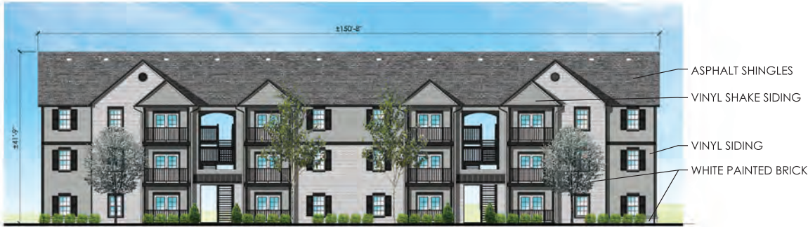
① TYP. 3 STORY CLASSIC BUILDING 'J' - FRONT ELEVATION SCALE: 1"=10'
