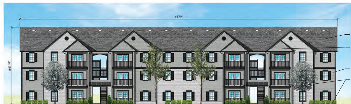
① TYP. 3 STORY CLASSIC BUILDING 'G' - FRONT ELEVATION SCALE: 1" = 10'
