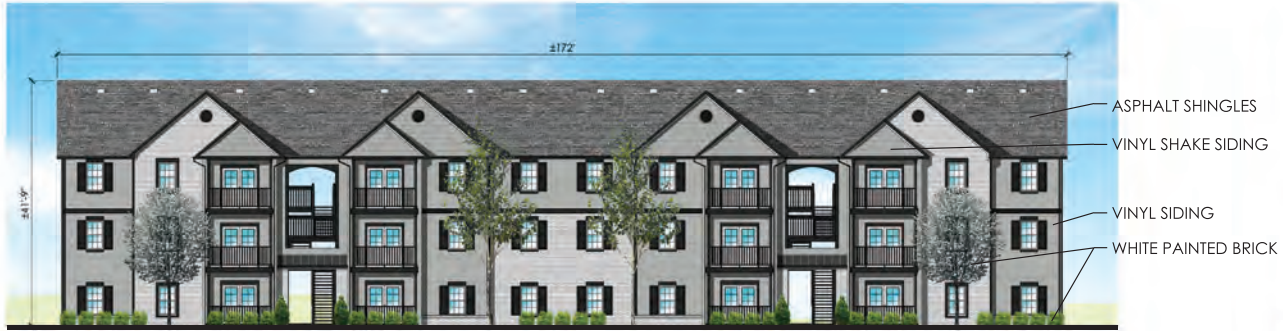
① TYP. 3 STORY CLASSIC BUILDING 'G' - FRONT ELEVATION SCALE: 1"=10'
