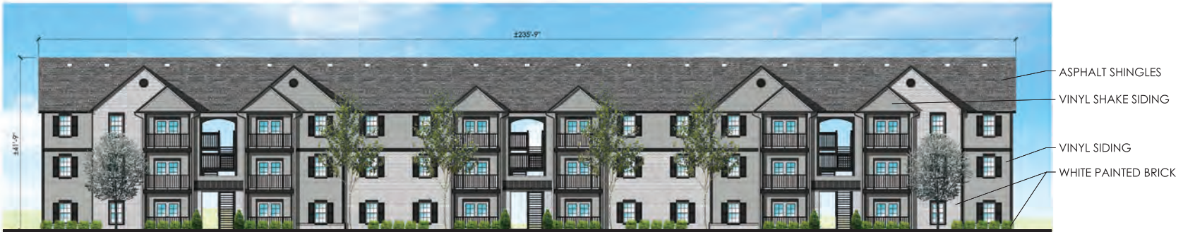
③ TYP. 3 STORY CLASSIC BUILDING 'K' - FRONT ELEVATION SCALE: 1"=10'
