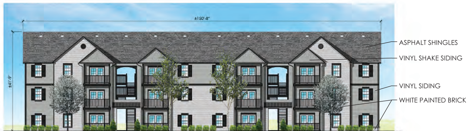
1 TYP. 3 STORY CLASSIC BUILDING 'J' - FRONT ELEVATION SCALE: 1"=10'
