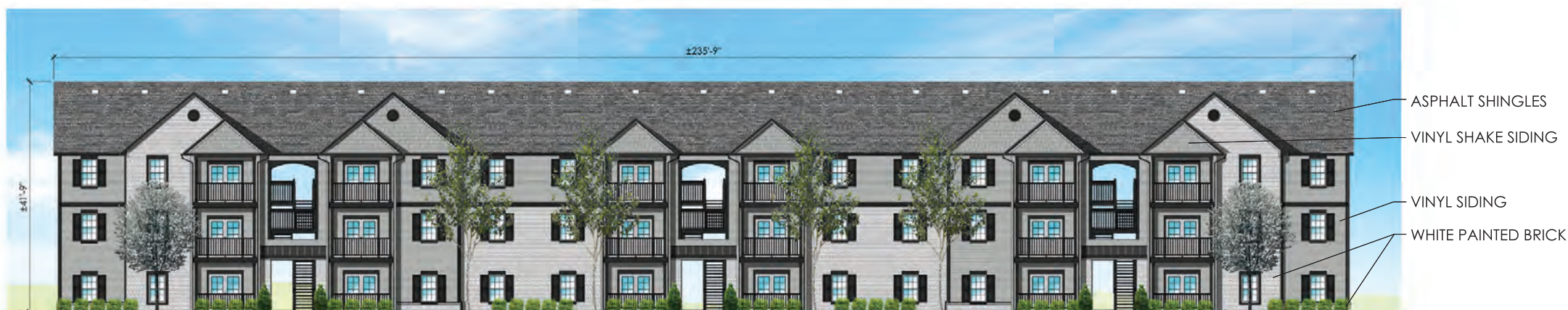
3 TYP. 3 STORY CLASSIC BUILDING 'K' - FRONT ELEVATION SCALE: 1"=10'
