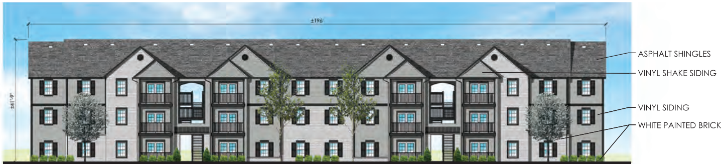
③ TYP. 3 STORY CLASSIC BUILDING 'L' - FRONT ELEVATION SCALE: 1"=10'
