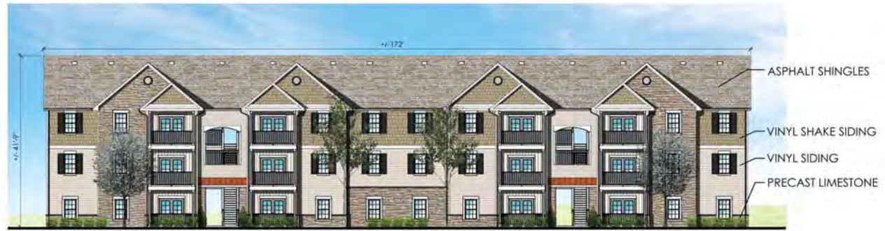
1 3 STORY BUILDING - 2 BED/2 BATH & FRONT ELEVATION SCALE: 1"=10'
