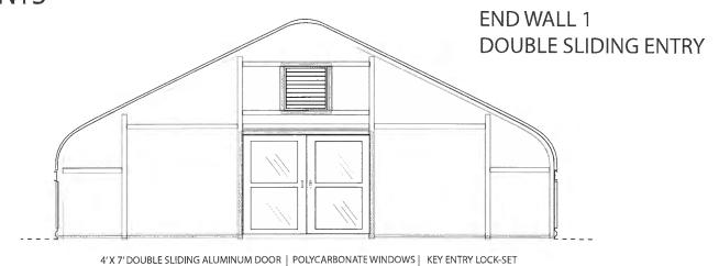
30" X 30" ALUMINUM SHUTTER | SOLAR WAX TUBE OPERATED
