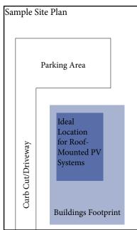
PV System should be flat against the roof of the historic structure or arranged so that the height of the system is not intrusive.
